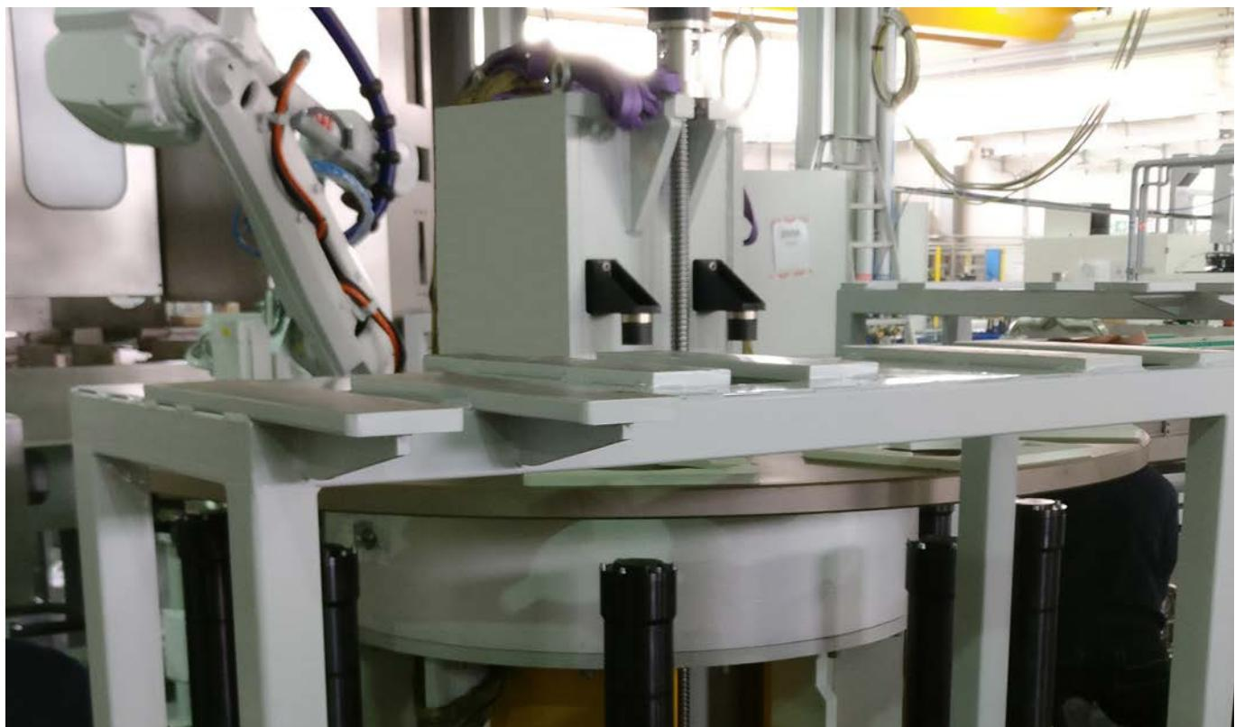
TIG 1200 HD - Automation bearing induction hardening process
