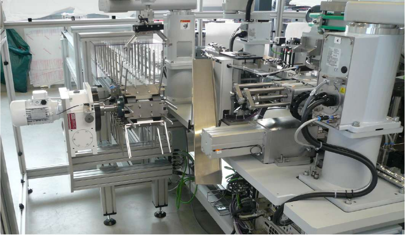
PBC 80 x 1000 mm - Drawer guides assembly
