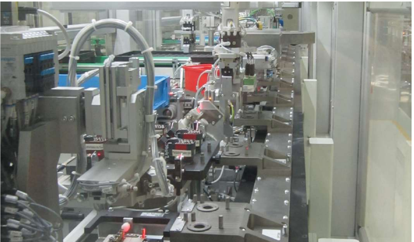
PLC HA 5.5 x 196" - Pencil ignition coils assembly
